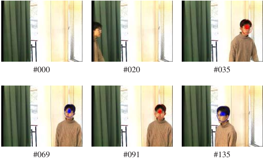
Fig. 15.14. Examples of detected human heads (colors means orientations).
