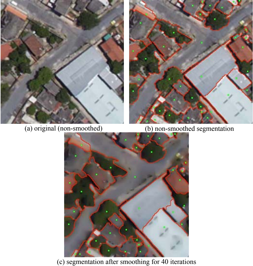
Figure 5. Effect of denoising on ISS segmentation, aerial image.
