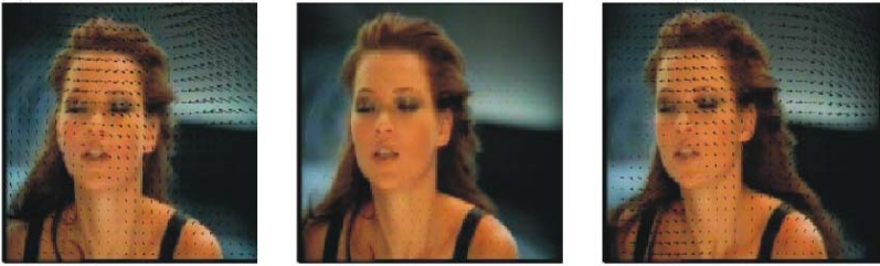
Fig. 1.6. Three frames of a sequence of five images, where 3 eigenvectors of appearance and a polynomial model of 4^{th} degree have been used to the registration process. Right side image shows the estimated optical flow respect to the middle frame (which corresponds to the third one in the sequence). Left side one is the computed optical flow respect to the middle one.
