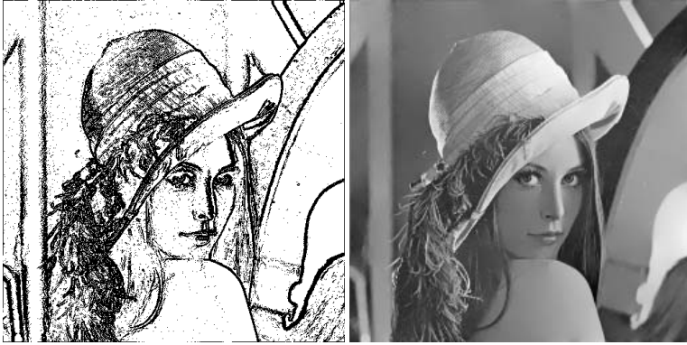
Fig. 3.6. Left: MSM with Lorentzian wavelet, h_\infty = -0.5 \pm 0.2 . Right: reconstructed image (PSNR=24.52 dB).
