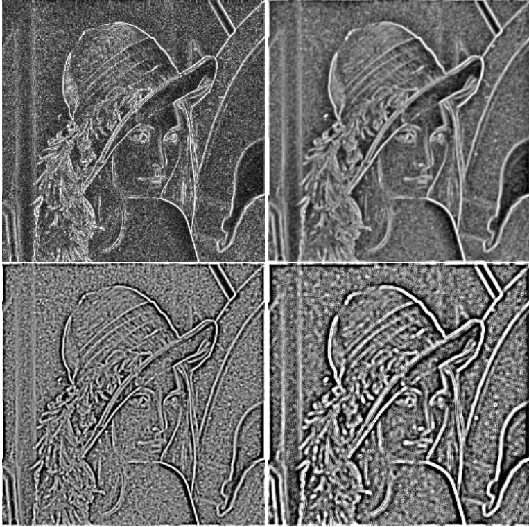
Fig. 3.2. Multifractal decompositions on Lena's image for Lorentzian wavelet and its derivative (top) and Gaussian wavelet and its second derivative (bottom) (see Section 3.5). The smaller is the singularity exponent, the brighter is the point.
