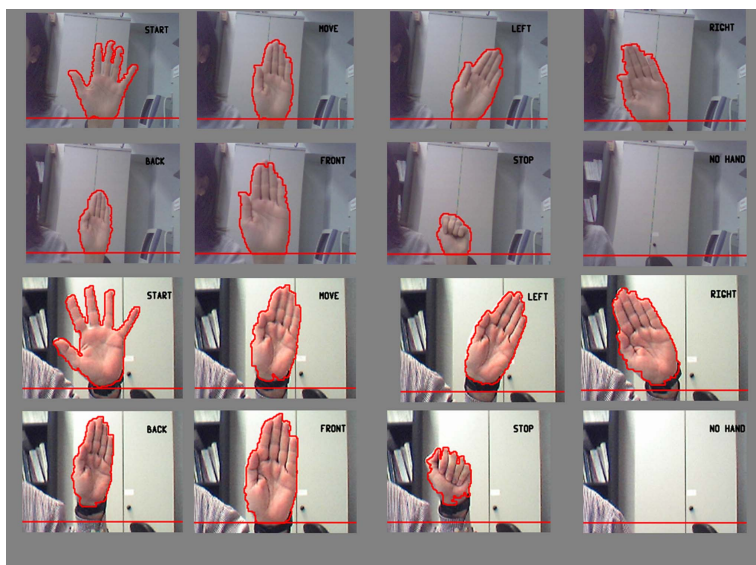
Fig. 22.5. Gesture recognition examples for different lighting conditions, users and hand configurations.
