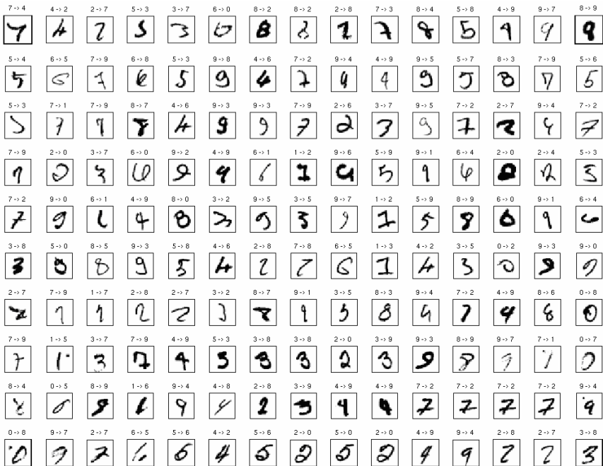
Figure 14. The 150 errors obtained on the test dataset (label -> decision).
